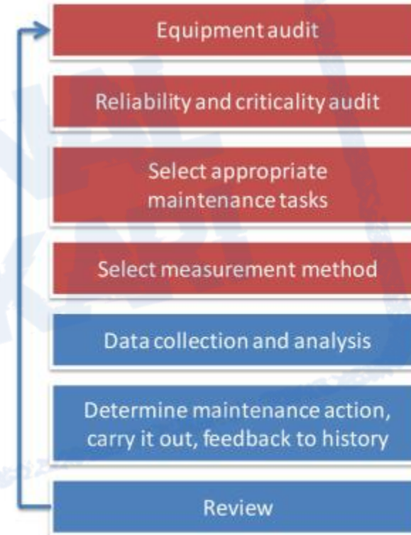
Figure 1-4 - ISO 17359: 2003 condition monitoring procedure flowchart
